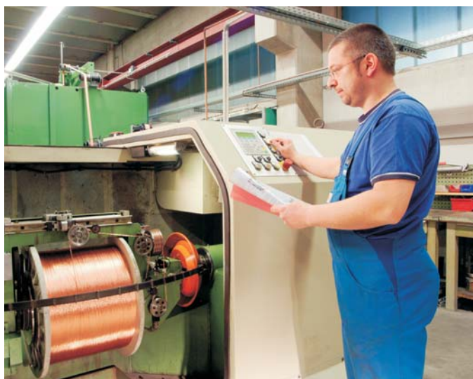
Twisting of conductors and manufacturing of round stranded cables
